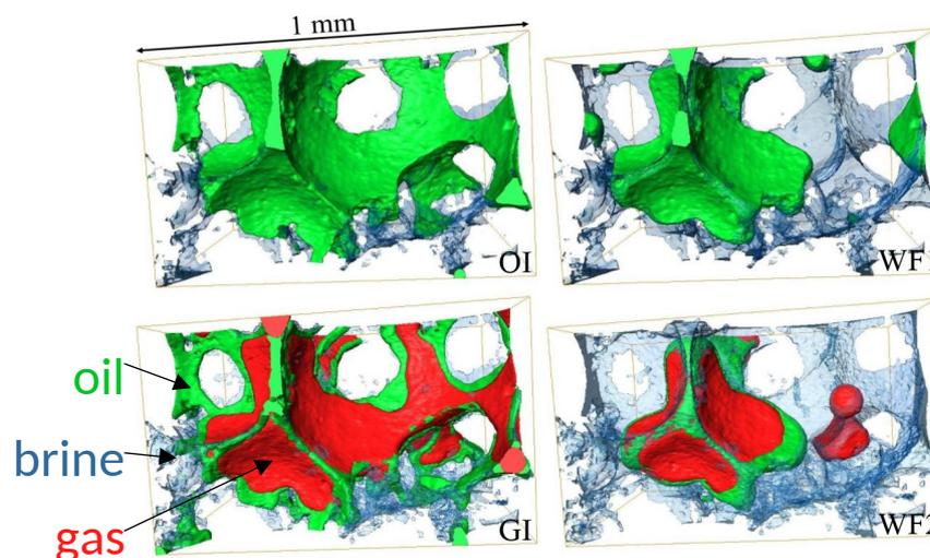
Figure 1: Three-dimensional visualisation of the arrangement of three immiscible phases - brine, oil and gas - in the pore space of a carbonate rock at high pressure and temperature. The four images are obtained at the end of oil injection (OI), first waterflooding (WF1), gas injection (GI) and second waterflooding (WF2).
