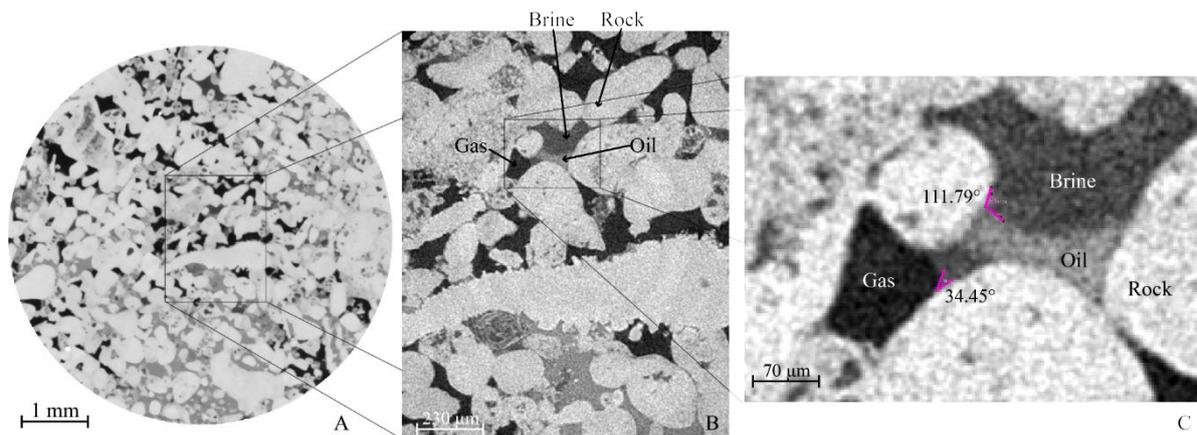
Figure 2: two dimensional slice of grey scale three dimensional images of the pore space obtained with micro-CT. We show how the change in wettability (quantified by contact angles) affects the arrangement of the fluids in the pore space.
