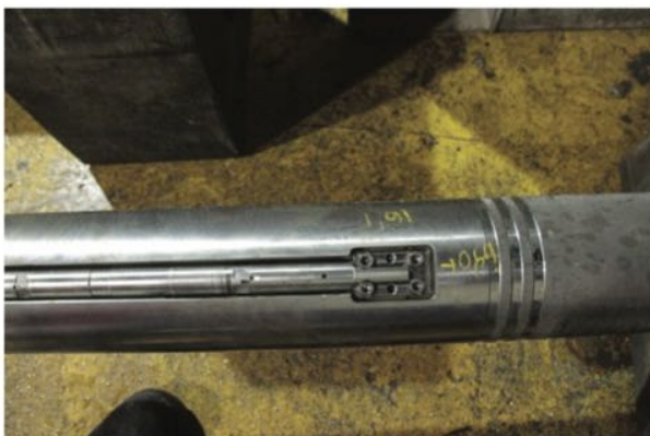
Gauge fitted inside a slot of a gauge carrier, ready to pick up and install in the DST string.
