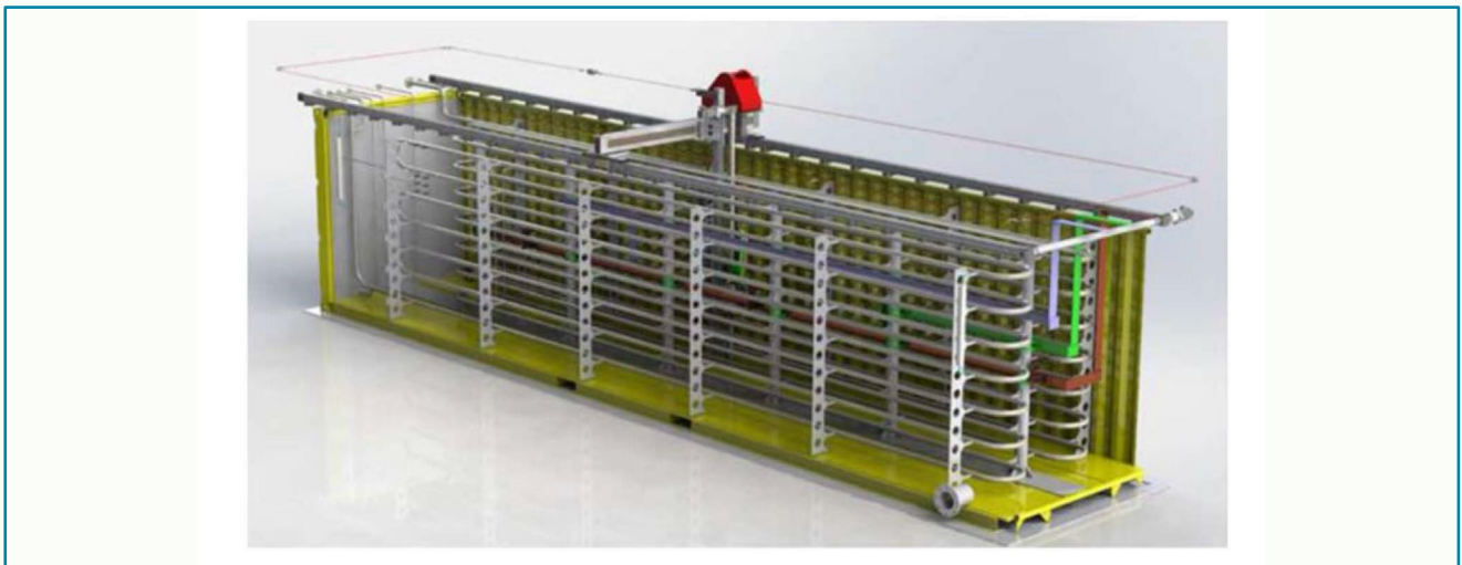
Figure 3. Container with the cooler pipes and the robot system used in the hydrocarbon flow loop tests.
