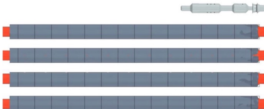
Figure 10—Cementing simulation outcome, with the tool at the end position of Figure 6. The dark grey color indicates that the cement volume fraction is above 95%.
